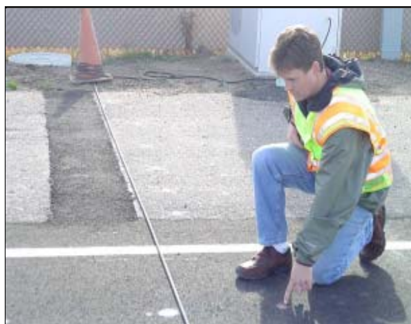
Minnesota's DOT Road Operations Engineer, Ben Worel, inspects one of the test cells made of taconite rock.
